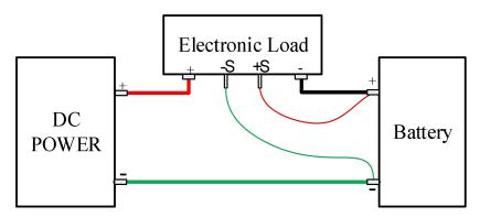
Figure 5-29 Charge Test Wiring Diagram
