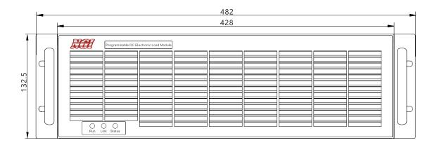
Figure 4-4 Slave Front Panel Dimension (mm)
