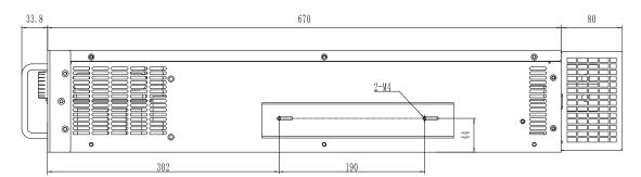
Figure 4-2 Side view dimension (mm)
