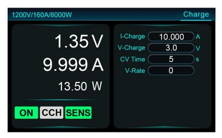
Figure 5-30 Charge Test
