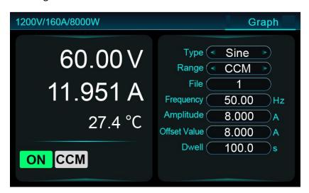
Figure 5-39 Dynamic Current Waveform
