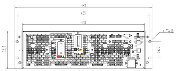
Figure 4-3 Rear panel dimension (mm)
