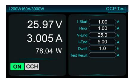
Figure 5-36 over-current test
