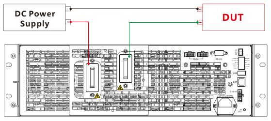
Figure 3-2 Low Voltage Operation
