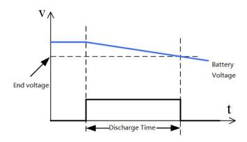
Figure 5-27 Discharge test curve
