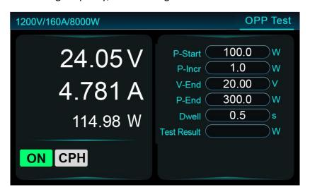
Figure 5-34 Over-power test
