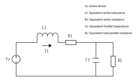
Figure 5-42 Impedance simulation
