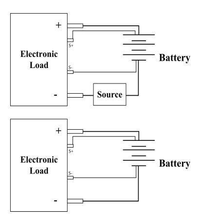
Figure 3-7 Discharge/Charge Connection
