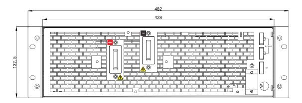
Figure 4-6 Slave Rear Panel Dimension (mm)
