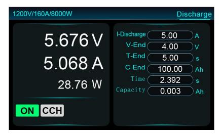
Figure 5-28 Discharge test
