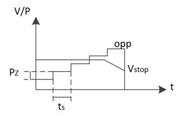
Figure 5-33 Over-power test
