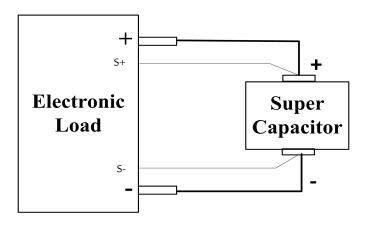
Figure 3-6 Super Capacitor DCIR Connection
