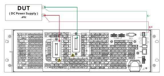
Figure 3-1 Sensing Connection
