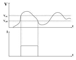
Figure 5-48 Latch Von onload and Voff offload
