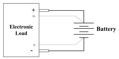
Figure 3-5 Battery DCIR Connection
