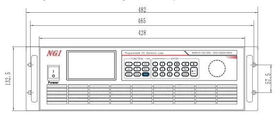
Figure 4-1 Front panel dimension (mm)
