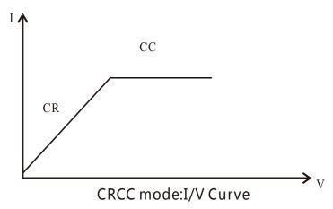
Figure 5-14 CRCC working curve
